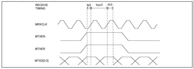
FIGURE 7-6: MAC MODE MII TIMING - DATA TRANSMITTED FROM MII
