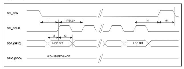
FIGURE 7-10: SPI OUTPUT TIMING
