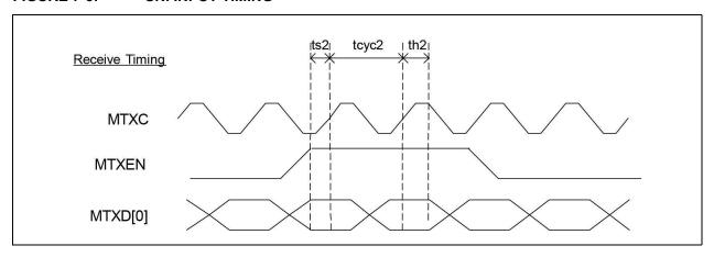
FIGURE 7-4: SNI OUTPUT TIMING
