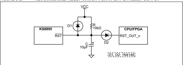
At power-on-reset, R, C, and D1 provide the necessary ramp rise time to reset the device. The reset out RST\_OUT\_n from CPU/FPGA provides the warm reset after power-up.
